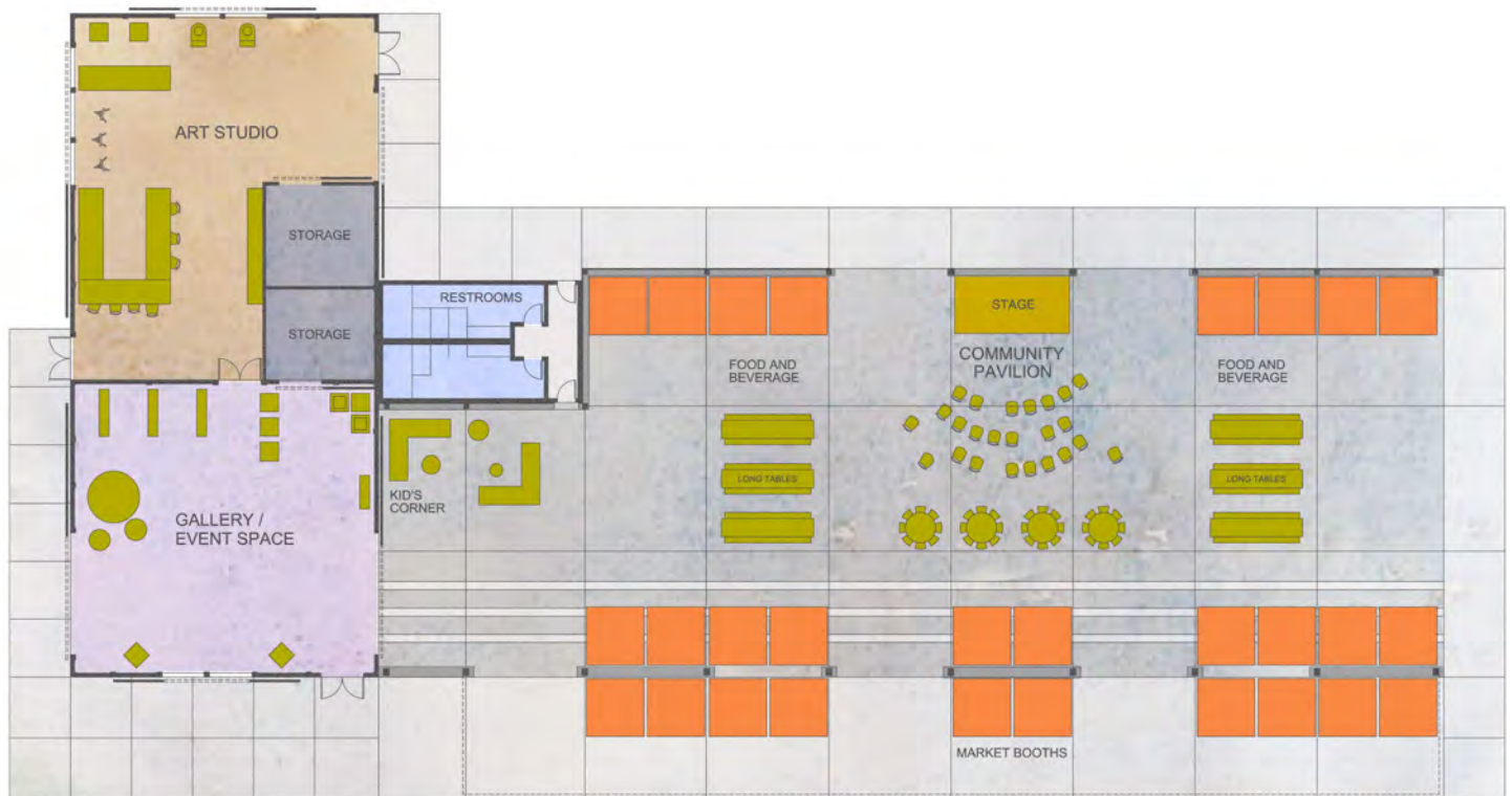
Fig. 3.4 Proposed plan for renovation of the Planer Shed
