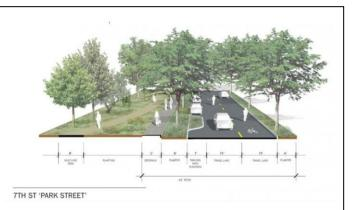
The future 7<sup>th</sup> Street Extension is in the planning and preliminary design stages. The proposed street design is shown in the picture above. It includes parking, street trees, sidewalks and trail alongside the river that intersects with 7<sup>th</sup> Street at various points along its route. The full design of these local street networks can be seen at the survey link or by coming to the open house.
