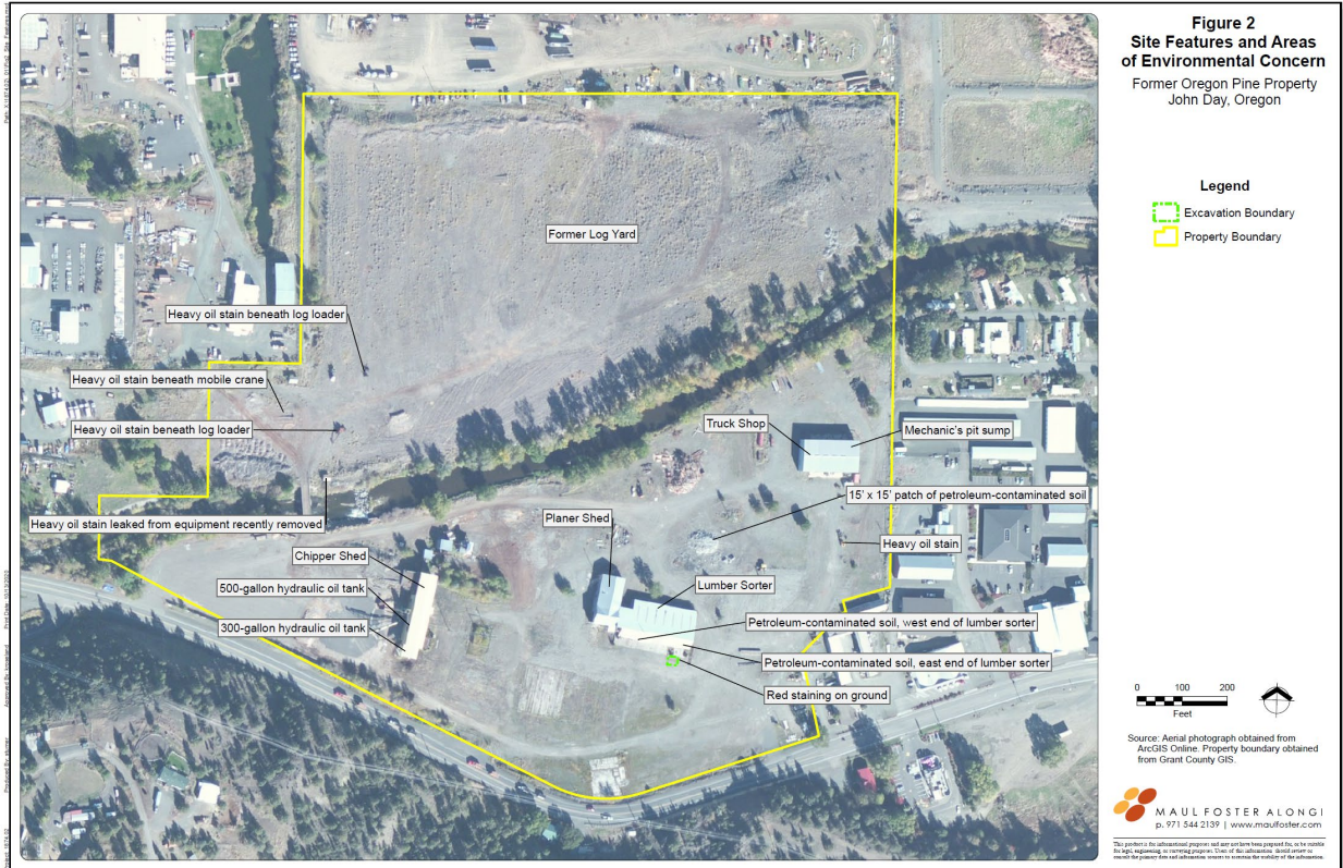
Figure 4. Site Features and Areas of Environmental Concern assessed by Maul, Foster, and Alongi, LLC
