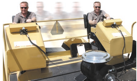
Sliding operator station provides the visibility and control to increase operating efficiency and reduce fatigue. Available with manual or powered control.
