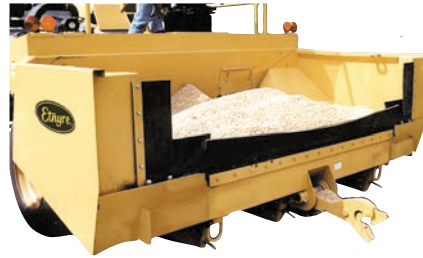
Folding Bat Wing Rear Receiving Hopper provides increased aggregate capacity and easy clean out of hopper. Facilitates easy change of aggregate types.
