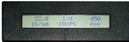
Computer maintains a uniform aggregate application even during changes in road speed. Stores five different application rates.
