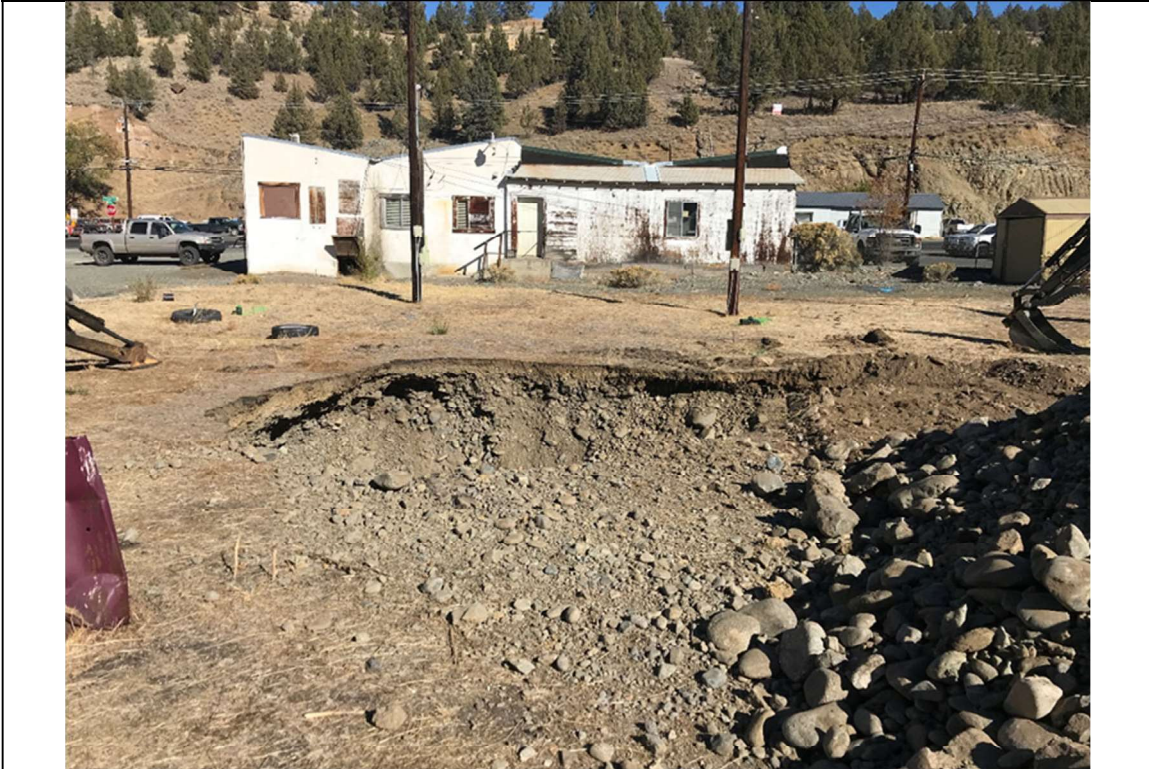
Photo 1. Infiltration test pit completed in October 2020 (looking east). Grant County Soil and Water Conservation District building is in the background. Note the thin layer of finer-grained material on top of coarse-grained material. The pile of cobbles in the lower right portion of the photograph is material removed from the test pit.
