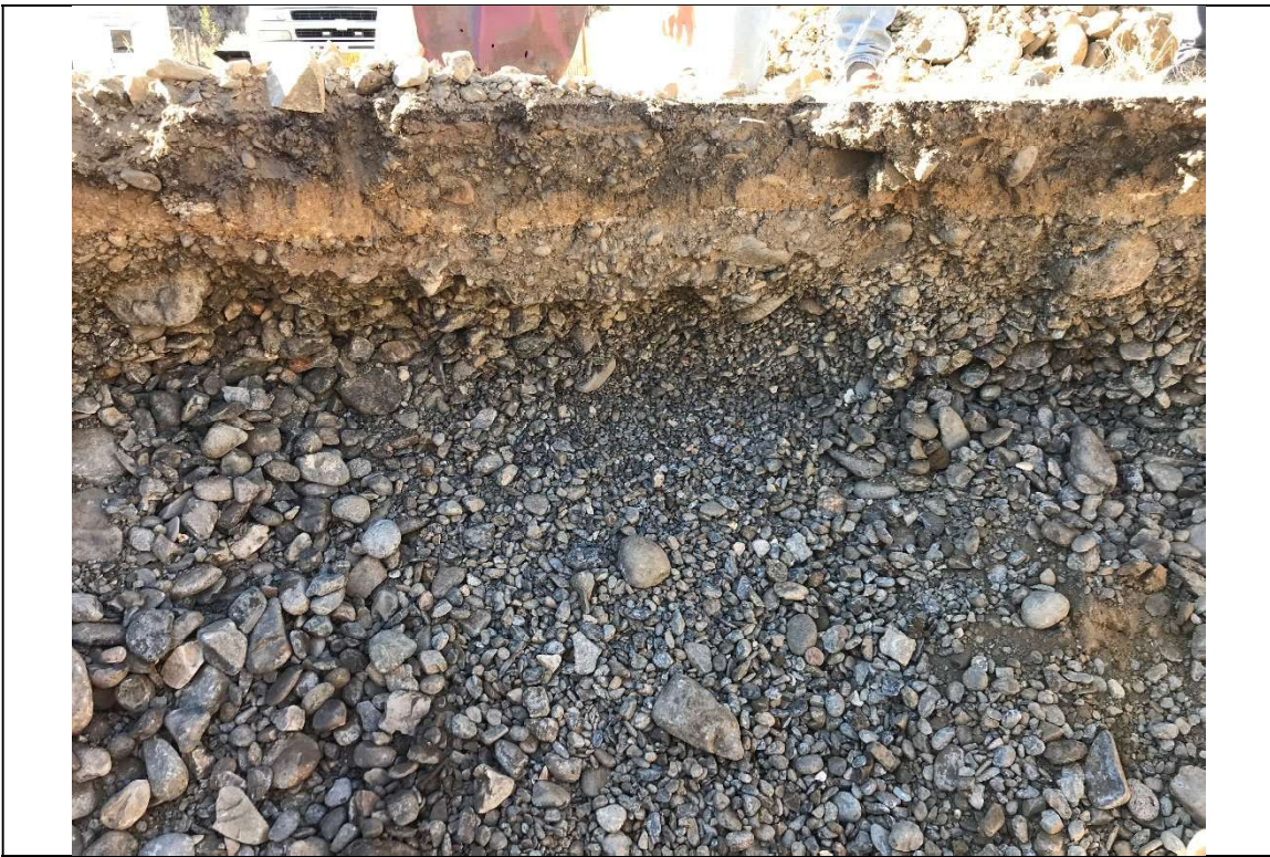
Photo 4. Profile view of the infiltration test pit showing the finer-grained materials at the surface.
