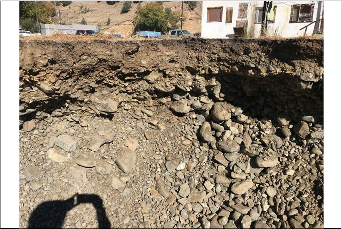
Photo 3. Profile view of the infiltration test pit showing the finer-grained materials at the surface.
