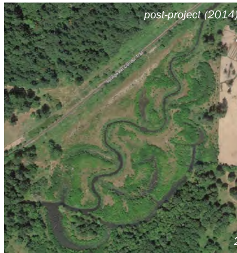
Johnson Creek Schweitzer Natural Area Project in Portland, OR. In the 1930s, the stream was straightened, ditched, and lined with stone armoring. The project re-created a meandering pattern, created pools and riffles, added large wood for habitat, and created off-channel alcoves, wetlands, and side channels. The project also included extensive planting of native vegetation and excavation of material to lower and reconnect the floodplain, which could potentially be used in the City of John Day to accomplish multiple ecological and human objectives.
