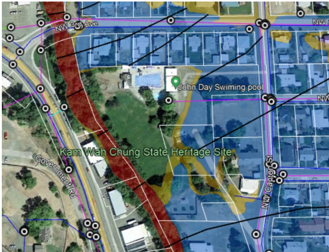
Figure 1. Flood Maps for Gleason Park and Pool, effective October 17, 2019. 100-year floodplain shown in Blue.
